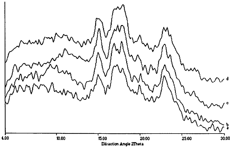
Fig. 9. X-ray diffraction patterns of wheat starch ionic starch ethers: microwave assisted reaction amphoteric derivative (a); rotating roaster reaction amphoteric derivative (b); microwave assisted reaction anionic derivative (c); rotating roaster reaction anionic derivative (d).
