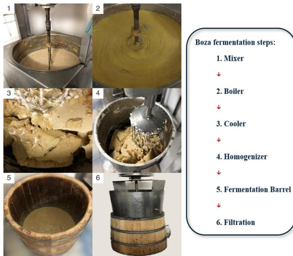
Figure 1. Schematic presentation of Boza fermentation procedure
